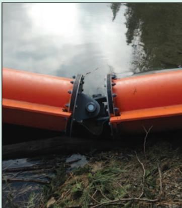
*The articulating universal joint connection of the multipurpose boom, which prevents axial roll while allowing articulation.*
